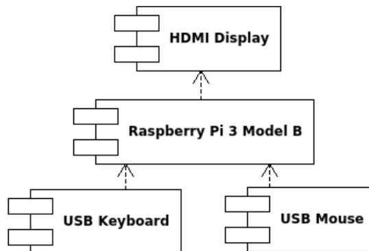
**Figure 7:** Component diagram of client log-in module
