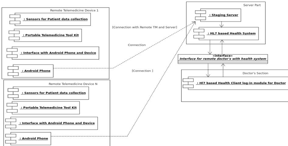
**Figure 8:** Deployment diagram of proposed telemedicine model
